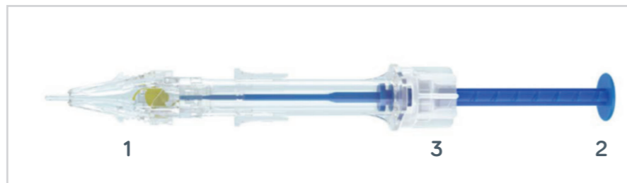
Figure 3: Note: 1, the insert shield positioned on the outside of the cartridge, to control penetration depth; 2, the plunger for push mode; and 3, the rotational knob for screw mode.
